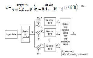
Fig. 1. Block diagram of selective mapping (SLM) technique for PAPR reduction.
